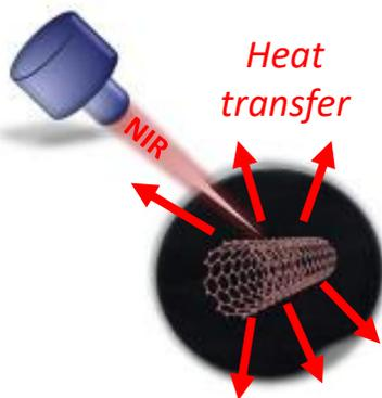
**Figure 2.** Schematic representation of photo-thermal heating by SWNT.
