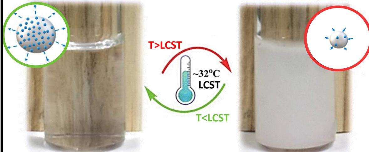
**Figure 1.** Schematic diagram of phase-transition behavior of PNIPAM. [Edited from: 1]
