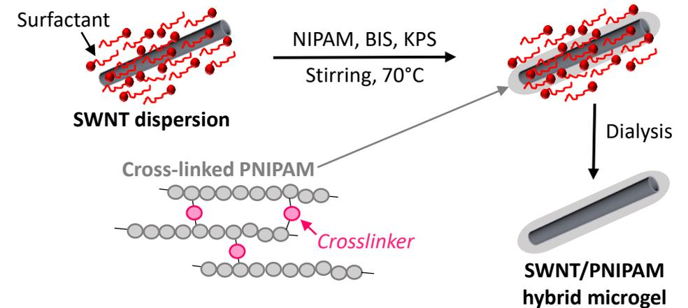
**Figure 3.** Schematic illustration showing the synthesis of PNIPAM/SWNTs hybrid microgels.
