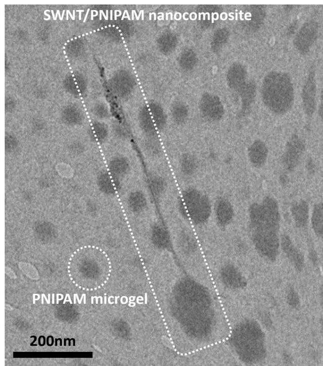
**Figure 5.** Transmission electron microscopy (TEM) picture of SWNT/PNIPAM hybrid microgels particles.
