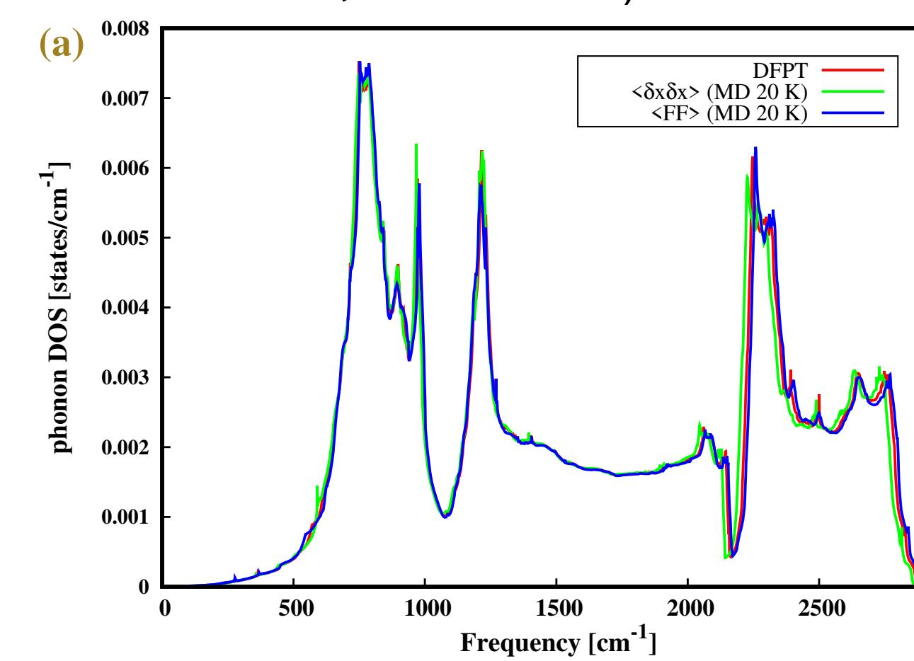
(a) Total phonon DOS from classical MD simulations at 20 K compared with DFPT calculation (red); (b) Total phonon DOS from PIMD simulations at 20 K compared with DFPT calculation (red).
