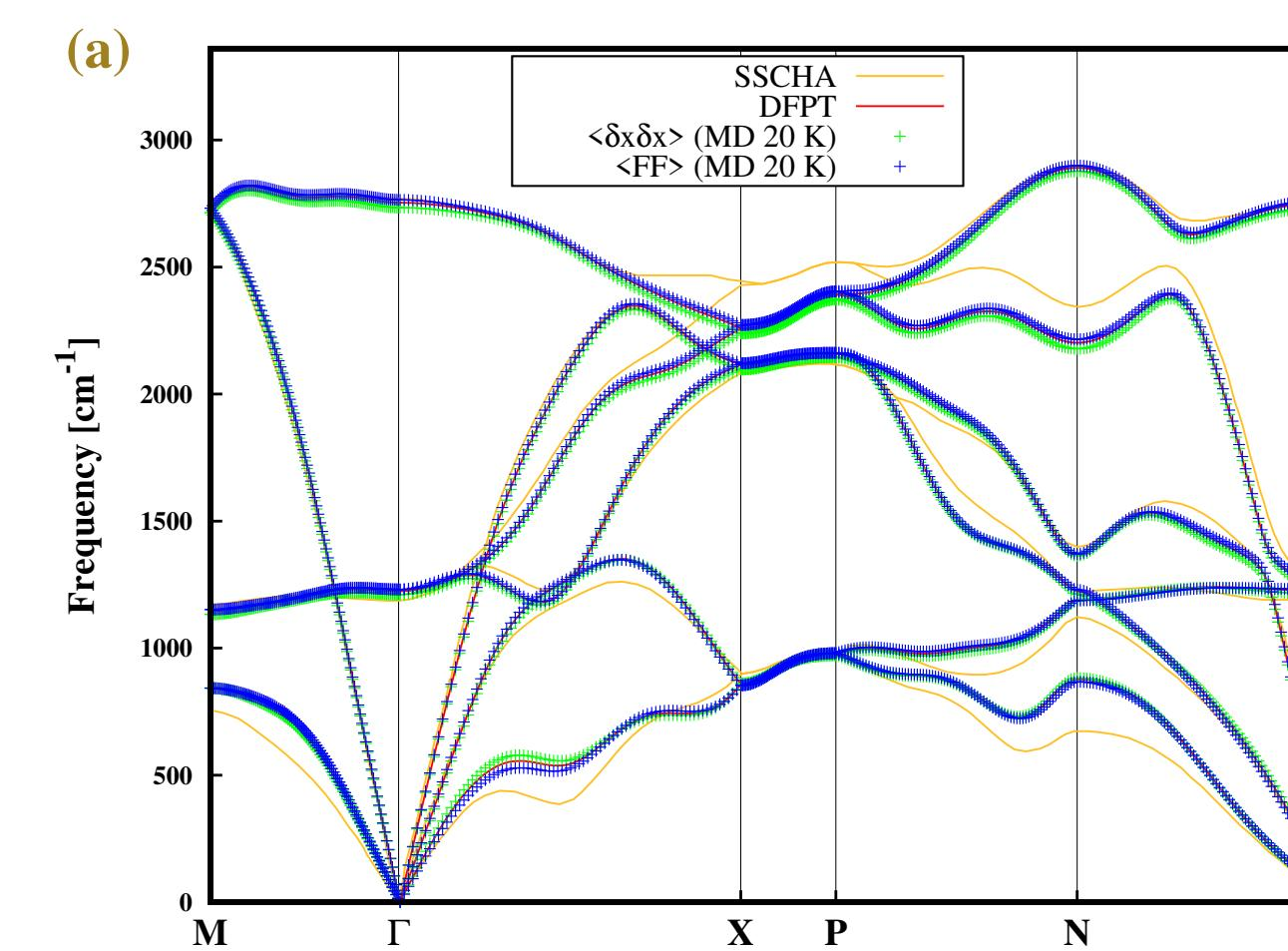
(a) Phonon dispersion from classical *ab-initio* MD simulations (PES evaluated at DFT level with PBE functional) at 20 K compared with DFPT calculation (red) and SSCHA (yellow). Red curve is perfectly covered by the force-force phonon estimator (blue). (b) Phonon dispersion from *ab-initio* PIMD (same PES as classical MD; 120 beads) simulations at 20 K.
