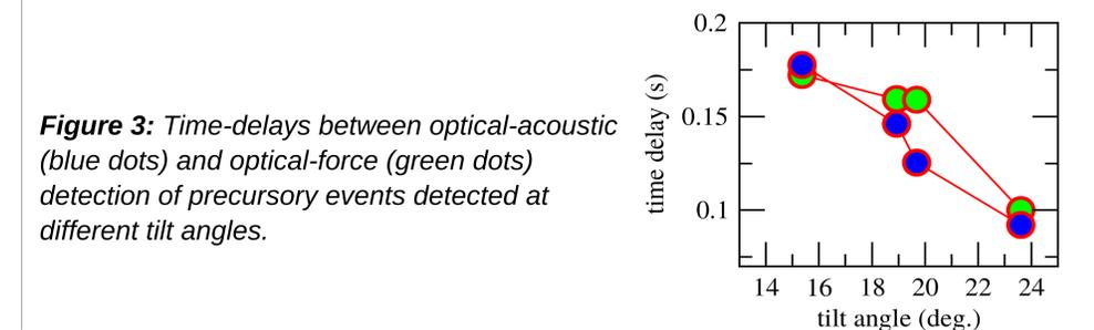
**Figure 3:** Time-delays between optical-acoustic (blue dots) and optical-force (green dots) detection of precursory events detected at different tilt angles.
