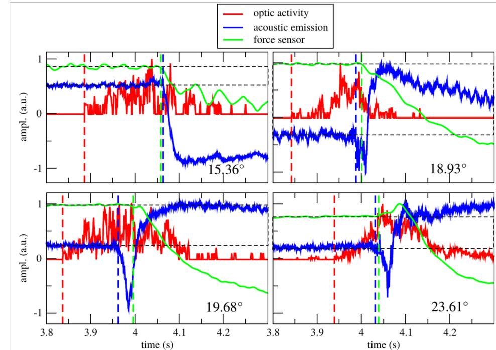
**Figure 2:** High-speed optical (red), acoustic (blue) and force (green) measurements during a precursory event with the associated starting times (dashed lines)
