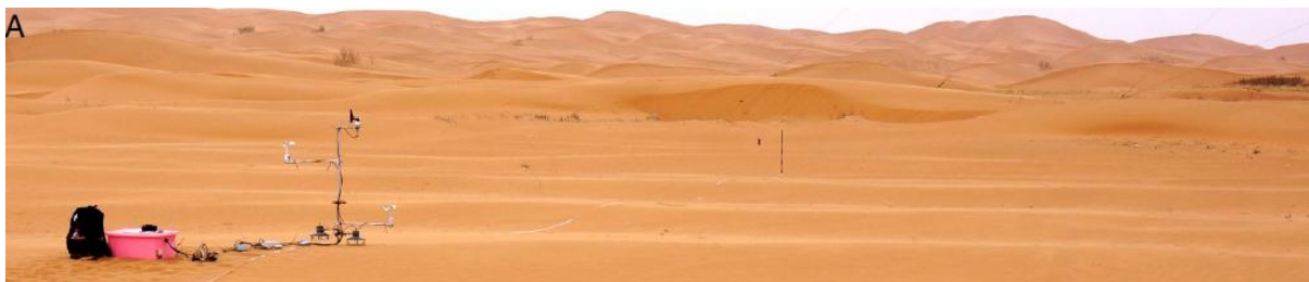
Fig. The mobile anemometer mast and incipient dunes.
